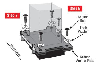
**Step 9:** Snug tighten the five anchor bolts, then check goal assembly with a level and inspect visually to determine if it is parallel and plumb to the playing surface.
