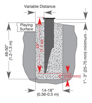
TIME OUT TIP: If you plan on mixing concrete in stages, work quickly to minimize time between batches.
