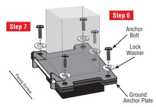
**Step 8:** Snug tighten the five anchor bolts, then check goal assembly with a level and inspect visually to determine if it is parallel and plumb to the playing surface.
